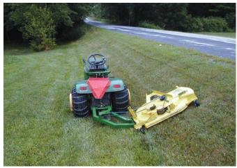
Needing to mow steep ditches along a busy highway near his place, Dave Braun built this ditch mower out of a spare riding mower deck.
