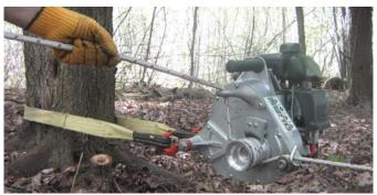
Portable Rope Winch is secured to a tree or other solid object using a polyester sling.
