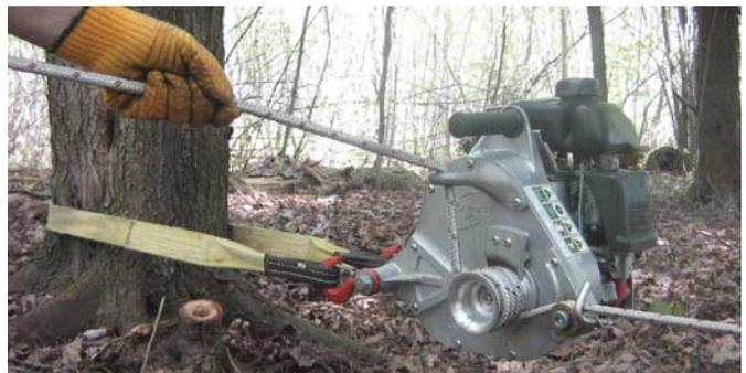
Portable Rope Winch is secured to a tree or other solid object using a polyester sling.
