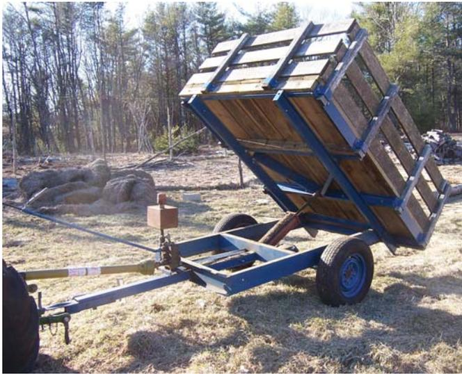
Steve Siter uses the pto-powered hydraulic pump off a 1937 dump truck to raise and lower his home-built dump trailer.
