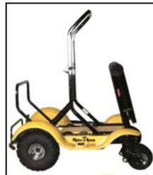
Mobili-T-Rover is driven by the wheels of an electric-operated wheelchair, which friction-drives 2 sets of large rubber rollers.
