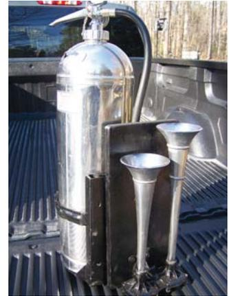
To scare away birds, Bill Jones made this loud air horn out of a 2 1/2-gal. fire extinguisher and a pair of air horns off an old fire truck.
