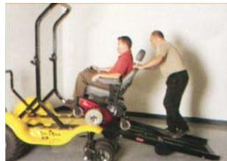
Operator drives wheelchair up a ramp on back until the wheels are between the rollers.
