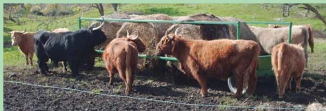
Feeder's open sides can be adjusted up or down, depending on the size of the animals and the bales.
