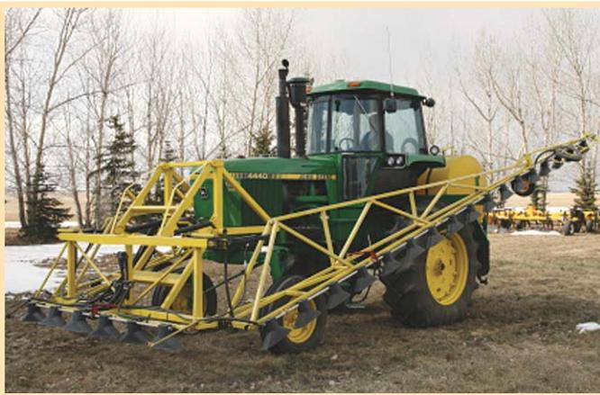
Robert Petrukovich converted a high clearance Deere 4440 tractor into this self-propelled sprayer, designing a mount that works like a front-end loader.
