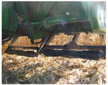
Kitchel stalk roller is designed to reduce stubble wear on tires and other equipment. Multiple 44-in. long sections each crush 2 rows of stubble.
