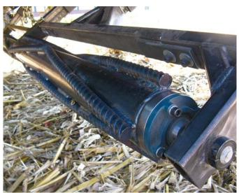
Spring tension presses stalks down and crushes them. Wrap-around rebar cleating enhances ground action of roller.
