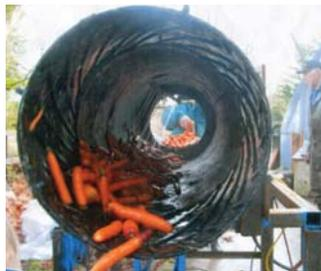
Water is sprayed onto vegetables as they feed through the rotating drum.
