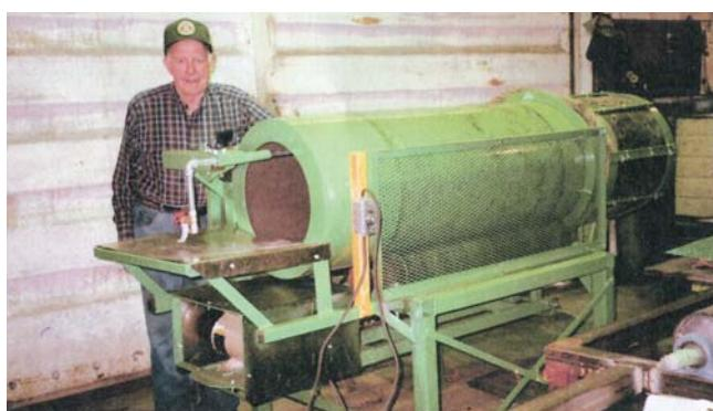
Belt-driven rollers turn the cleaner, with power supplied by a 3/4 hp electric motor.
