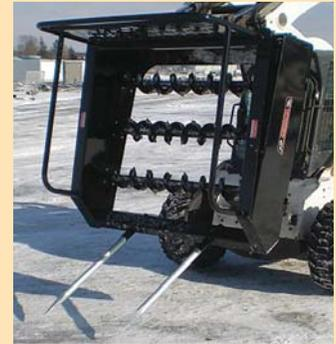
**Hydra-Shredder chops and spreads bales for bedding. Forks pick up bale, then unit is tipped back so bale rests on augers. Chopped straw then falls through to the ground.**
