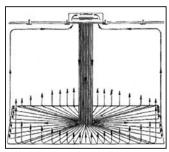
Vortex circulating fan keeps the temperature balanced in a room by gathering warm air near ceiling and forcing it to the floor in a 2-ft. dia. column of air.
