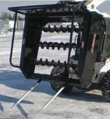
Hydra-Shredder chops and spreads bales for bedding. Forks pick up bale, then unit is tipped back so bale rests on augers. Chopped straw then falls through to the ground.
