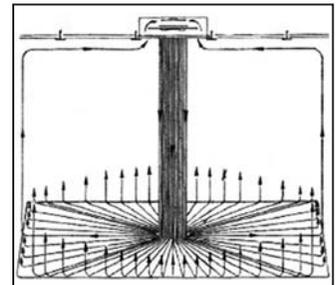
**Vortex circulating fan keeps the temperature balanced in a room by gathering warm air near ceiling and forcing it to the floor in a 2-ft. dia. column of air.**
