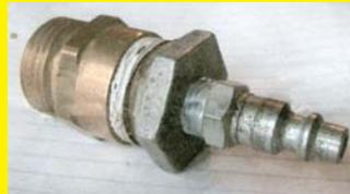
My neighbor, Lori Reichard, made up this little gadget, which does a fantastic job. I have two long runs of garden hoses to livestock tanks that always freeze up no matter how carefully I tried to drain them after filling tanks. Now I just screw this little gadget onto the end of the hose and attach it to an air compressor. It will blow a 100-ft. hose dry in about 30 sec. It requires about 125 psi to do a good job. **(Jim Cole, Ottawa, Kan.)**
