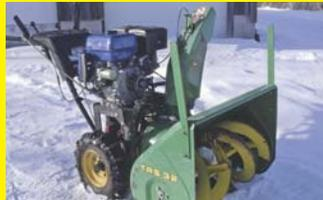
The drive unit on my Deere walk-behind snowblower kept breaking down. I replaced the drive with a hydrostatic unit from an Uber feed cart. A Cub Cadet transmission would also work. The frame of the snowblower was too small so I used 2-in. angle iron to build a platform to support the new drive unit. It worked great - lots of power. **(Phillip Krywosa, Boonville, N.Y.)**
