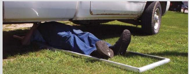
Creeper has a 4-ft. long movable bed that rolls on wheels inside an 8-ft. long metal frame. You just slide yourself under the vehicle.
