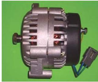
internal fans for superior cooling and heavy-duty roller bearings and long life brushes compatible with all the highly computerized systems found on most equipment today. It has 150 amps compared to 90 amps on Nippondenson-style alternators, which comes in handy for high amp demand like extra lights and electronics.
