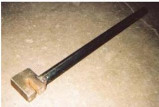
"I made this straightening tool out of a 1 1/2 by 3 by 4-in. chunk of steel with a 3/8 by 2-in. wide slot in it. I use the tool like a heavy pipe wrench to straighten or bend steel bars. To make the tool I milled the slot in, and then welded on a 1 1/4 by 36-in. steel pipe handle."
