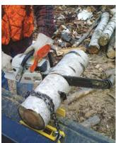
LogMaster attaches to loader bucket (left). Then you lay a log on top and strap it down with a chain to hold for cutting.
