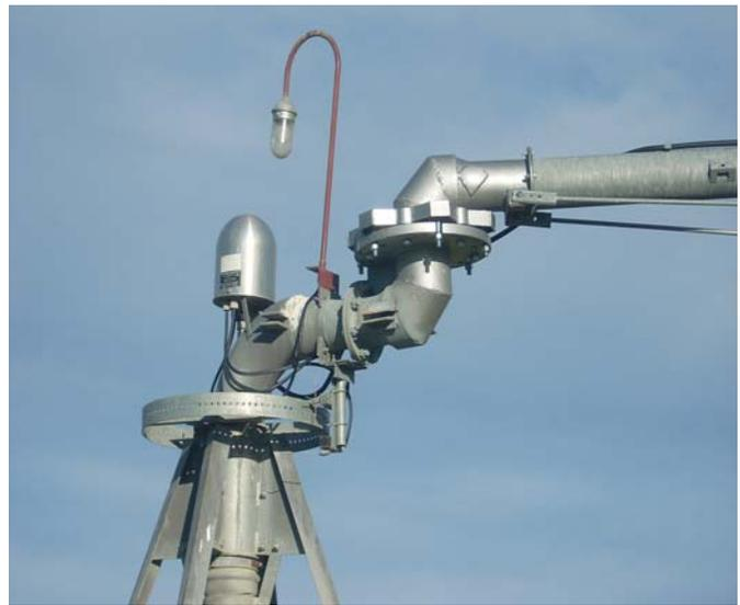
**Pivot Jetter moves pivot's wheels to fresh ground, before deep ruts are created.**
