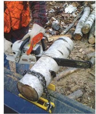
**LogMaster attaches to loader bucket (left). Then you lay a log on top and strap it down with a chain to hold for cutting.**
