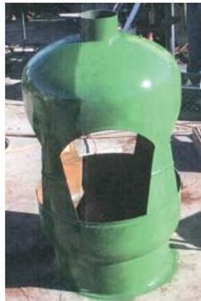
Openings cut into tank convert it to an outdoor fire pit.
