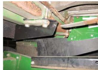
Between row deflector (left) and in-row deflector mount on the underside of chopper-style Deere corn heads, keeping trash from windrowing to the side.
