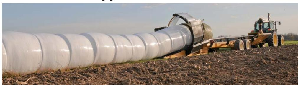
BaleLiner consists of a wrapper that piggybacks on a bale wagon for transit. Once the wrapper is unloaded, the wagon can pick up and haul up to 8 bales at a time and wrap them in the fields.
