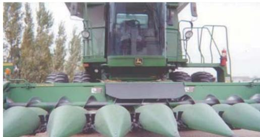
Grain Saver lays feeder house to prevent corn ears from bouncing out.
