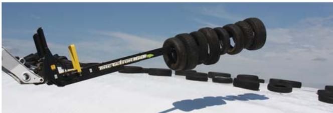
Tire Gator 160 slides onto standard pallet fork tines and is driven by tractor hydraulics.
