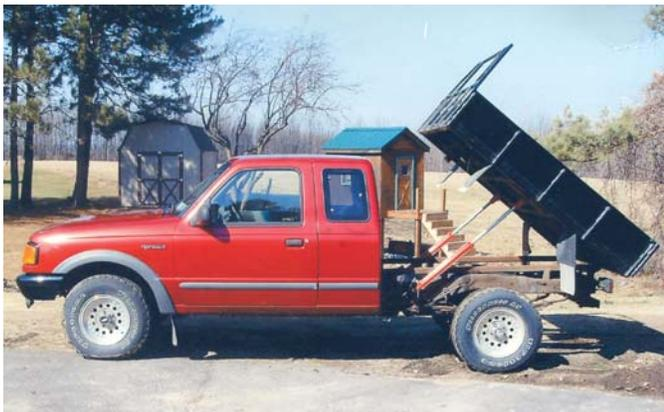
Danny Goodman and son Logan converted a 1993 Ford Ranger 3/4-ton, extended cab pickup, unbolting the pickup bed and replacing it with a home-built dump box.
