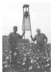
Electric fan mounts under light and blows bugs into 4-ft. nylon bag.
