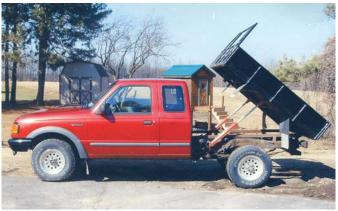
Danny Goodman and son Logan converted a 1993 Ford Ranger 3/4-ton, extended cab pickup, unbolting the pickup bed and replacing it with a home-built dump box.
