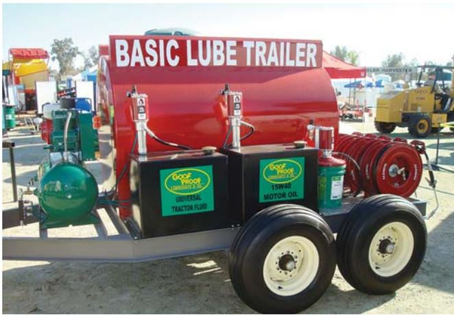
Basic Lube Cart has a 550-gal. double-wall fuel tank, a 40-gal. clean oil tank, a 40-gal. spent oil tank, a 5-gal. grease pail with a pump, and a 5 1/2 hp air compressor.
