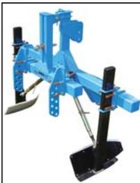
The Bedlocker is a toolbar with two sets of Teflon-surfaced skis. Skis lock toolbar-mounted equipment to bed sides for precision planting or cultivating.
