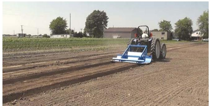
A machine called the Bedformer makes raised beds, allowing planting, cultivating, spraying and other tasks to be carried out with precision.
