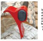
Axe head attaches to handle from the side, creating an off-line center of gravity (left). As axe strikes log it begins to incline, creating torque that multiplies the splitting force.
