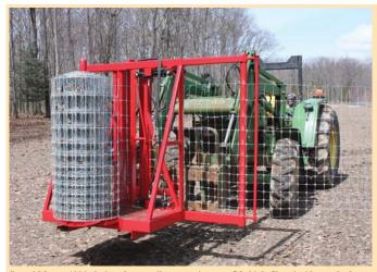
StretchMaster 100 is designed to unroll woven wire up to 5 ft. high. Since it rides on the frontend loader, it can be used to hang a second roll above the first for fences up to 10 ft. high.
