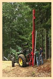
Extensions for the PostPounder (left) are available to drive posts up to 18 ft. long. The T-PostPounder (right) is a manual pounder that has a hinged opening on one side that makes it easy to place over post.
