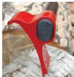
Axe head attaches to handle from the side, creating an off-line center of gravity (left). As axe strikes log it begins to incline, creating torque that multiplies the splitting force.
