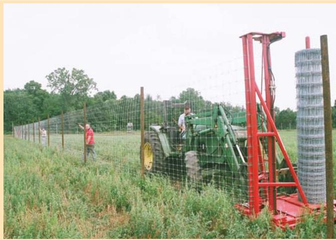
Optional attachments lets you put up rolls of wire up to 10 ft. high. Loading a roll of wire on to Beem's fencing units is easy. Just tip the front end loader down and spear the roll.
