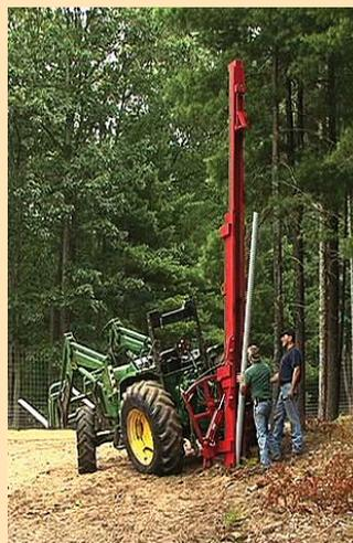
Extensions for the PostPounder (left) are available to drive posts up to 18 ft. long. The T-PostPounder (right) is a manual pounder that has a hinged opening on one side that makes it easy to place over post.
