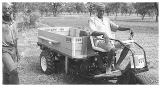
The Basic Utility Vehicle, or BUV, is a low-cost ATV without all the bells and whistles. It can be fitted with tractor-style tires for farming and logging.
