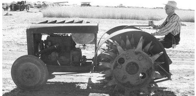
Spiked wheels on Fageol tractors were designed to "walk" over fields, without compacting the soil. But in reality, the wheels often dug down to the frame and spun hopelessly.
