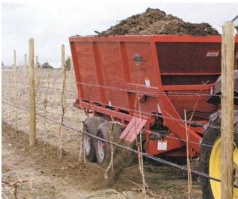
The Whatcom mulcher has a variable speed discharge belt that pours mulch material into rows. Deflector slats can be adjusted to vary row width.
