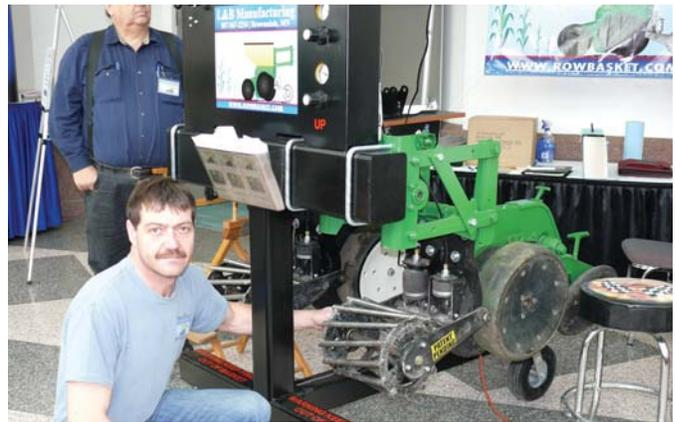
Rolling baskets can be raised and lowered separately from planter row units, just ahead of the openers. Air bags provide down pressure.
