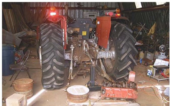
To split tractor, Gustafson installed a bale spike on the 3-pt. hitch, lowered it down to floor level, and put a weighted wood pallet over it.
