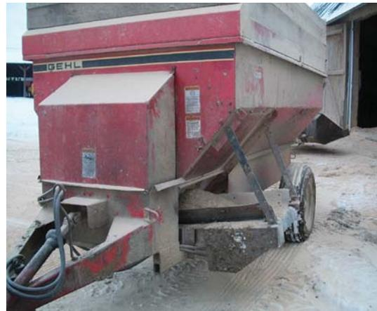
Conveyor belt on front of wagon is chain-driven by a hydraulic motor. Wood shavings drop down on belt and are shot out the side.
