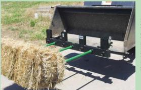
"Ultra fork" clamps onto loader bucket and comes with 7 replaceable, 32-in. long spears. Spears extend through holes in frame and are secured by lynch pins.
