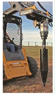
Offset cone makes auger wobble as it pushes into the ground. The result is a hole with no loose dirt in the bottom or around the top of the hole.
