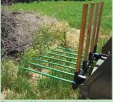
Top part of frame has 4 stake pockets to hold 2 by 4's that form a "backstop" when hauling brush.
