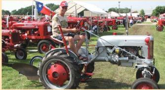
Gary Dotson repowered his 1948 Farmall Cub with a Kubota 4-cyl., diesel V-800 engine (above). Dotson built a new frame out of heavy steel plate for the engine to bolt to.
