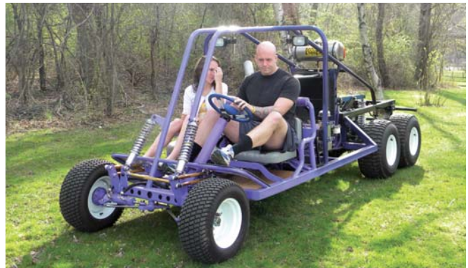
Built from a wide variety of parts, Macqueen's "dune buggy" is powered by a rebuilt Mitsubishi 4-cyl. diesel engine.
