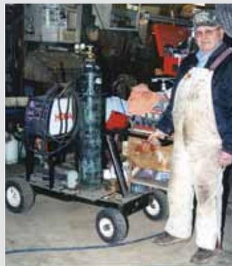
So I used the running gear and frame from an old riding mower to build a 4-wheeled welder cart.
