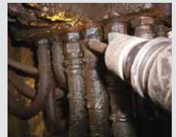
"To solve the problem, I used an air hammer and a punch against the sides of the fittings to break them loose. Then I used the same idea to retighten the new hoses. It took no time at all, and the new fittings don't leak a bit."
