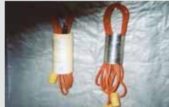
**Al Burant, Barrys Bay, Ont.:** "I find that cans or large pop bottles work well for storing long extension cords. I've used this idea for at least 30 years. I just coil up the cord and slip it into a can, which holds it tightly together."
