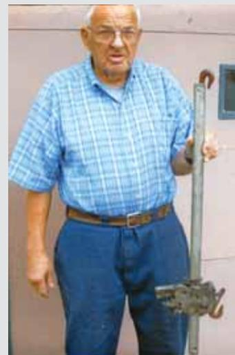
**Russell Delancy, Leavittsburg, Ohio:** "I made a cheap, heavy duty chain binder out of an old car bumper jack and two chain hooks. I removed the base from the jack, then drilled a hole into one end of the jack post and bolted a chain hook into place. Then I bolted another chain hook to the jack mechanism itself."
