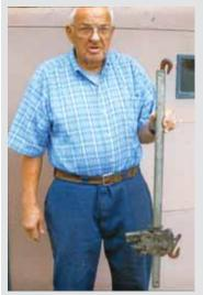
Russell Delancey, Leavittsburg, Ohio: "I made a cheap, heavy duty chain binder out of an old car bumper jack and two chain hooks. I removed the base from the jack, then drilled a hole into one end of the jack post and bolted a chain hook into place. Then I bolted another chain hook to the jack mechanism itself."
