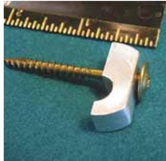
Wire fastener consists of a 1-in. long, 1/4-in. wide aluminum alloy clip (left) with a slot near the toe that holds the wire and a self-tapping torx head screw.
