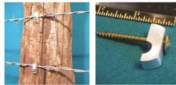
Wire fastener consists of a 1-in. long, 1/4-in. wide aluminum alloy clip (left) with a slot near the toe that holds the wire and a self-tapping torx head screw.
