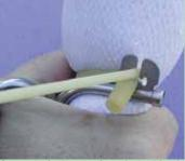
One end of a length of surgical tubing is inserted in the clip. Operator grabs other end of tubing and stretches it into place.
