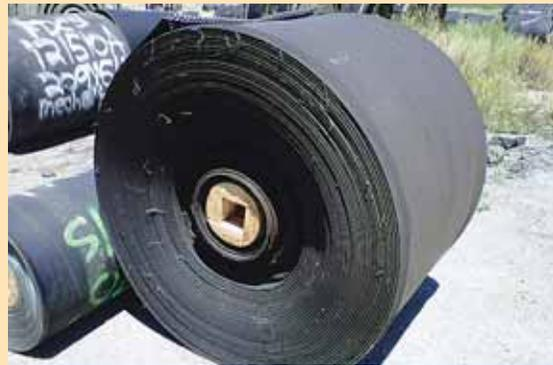
Rolls of heavy duty 4-ft. wide, 3/8-in. thick rubber conveyor belt work great for building windbreaks around livestock yards.
