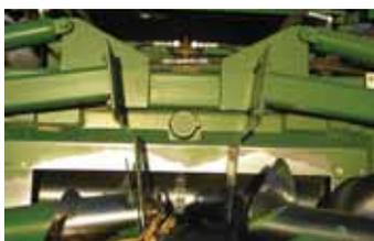
Header's 2 sides are anchored to a center pivot point allowing header to flex 18 in. up (left) and 15 in. down (right) from level.
