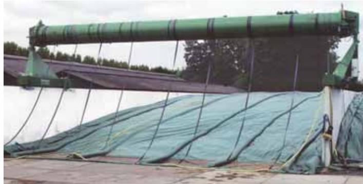
Self-winding reel rolls the length of the bunker, picking up the removable cover as it goes.
