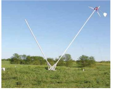
Roy Hershberger's 90-ft. windmill comes down fast for maintenance, with no need to loosen the 8 guy wires that support it.
