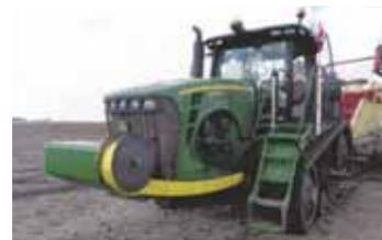
Cable runs back under tractor to a heavy duty pin with a cable pulley housed, inside a steel bracket bolted to tractor frame. Nylon strap pulling system is also available.
