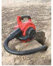
Gas-powered Cheetah uses a small engine and fan to push exhaust fumes into pest
