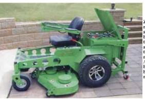
Zero turn mower uses a deep-cycle battery pack that provides an average 90 to 120 min. of mowing time. A replacement batter pack can be installed in 5 min. or less.
