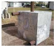
A 22-in. dia. door is cut into one end of stove for loading wood. A heat duct and cold air return are on back.
