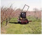
Machine uses 2-ft. long plastic strings evenly spaced along a rotating vertical spindle. As operator drives alongside trees, rotating strings knock off blossoms.
