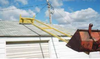
Loader-mounted snow rake extends 20 ft. out from bucket to cleara a 4-ft. wide area.
