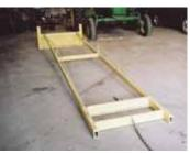
Rake's 3-ft. wide frame attaches to loader bucket using a pair of chains and binder.
