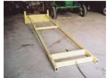
Rake’s 3-ft. wide frame attaches to loader bucket using a pair of chains and binder.
