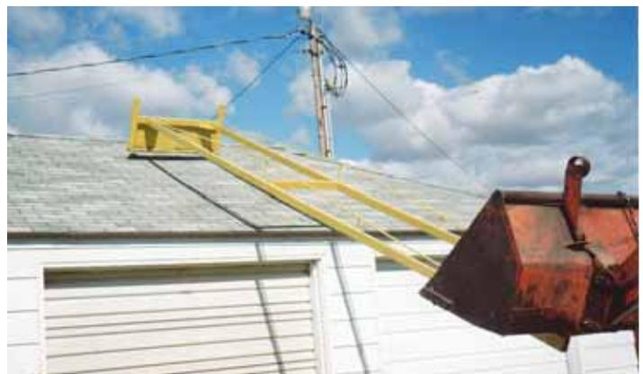
Loader-mounted snow rake extends 20 ft. out from bucket to clear a 4-ft. wide area.
