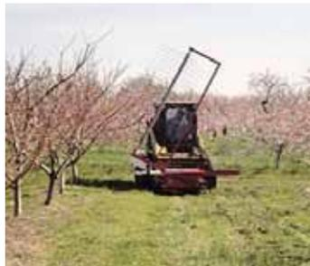
Machine uses 2-ft. long plastic strings evenly spaced along a rotating vertical spindle. As operator drives alongside trees, rotating strings knock off blossoms.
