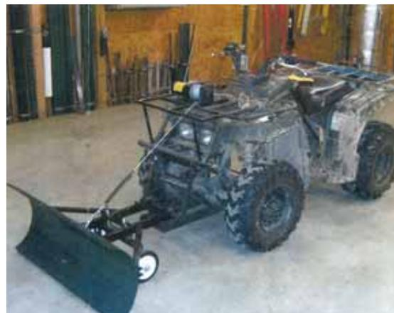
Snow blade is raised and lowered by an electric winch that's operated by ATV's 12-volt battery.
