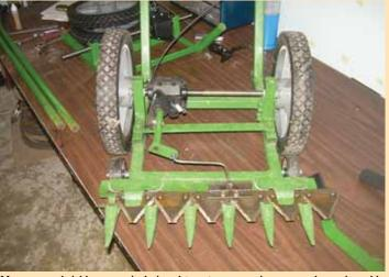
Man-powered sickle mower is designed to cut grass, grain crops and even brambles
