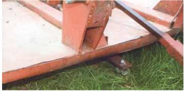
As seed falls through hole in deck, spring-loaded tines bolted to mower's flail arms
