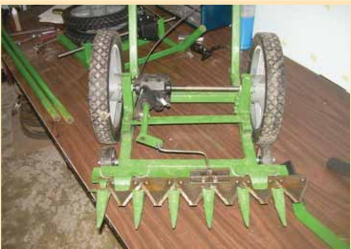
Man-powered sickle mower is designed to cut grass, grain crops and even brambles and light brush.
