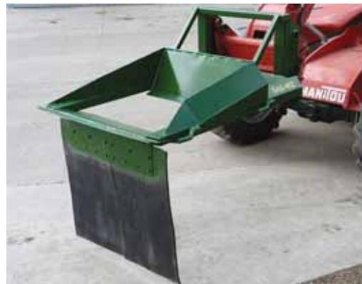
**Loader-mounted bagger digs into pile of firewood. Operator then flips unit back and tosses wood into bag until it’s full. Heavy-duty rubber flap protects front side of bag while loading.**
