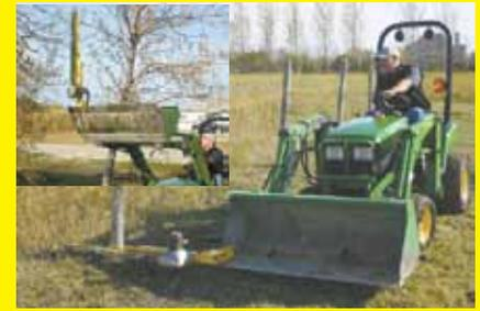
Hydraulic-powered cutter attaches to loader bucket.
