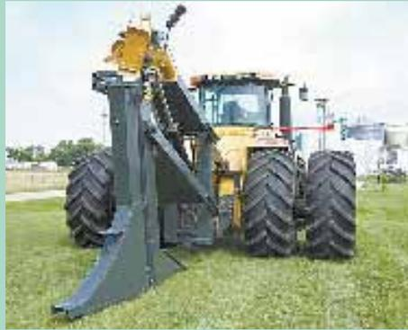
Interchangeable boots mount on quick-tach tile plow by simply pulling a single rod.
