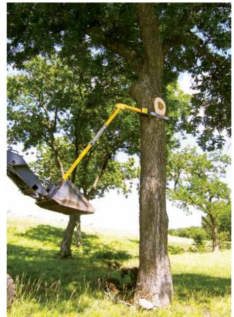
**Tree trimmer has an 8-ft. mast and mounts directly to receiver on front-end loader.**
